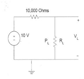
8. Use Matlab for finding nodal voltages of the circuit as shown below.
