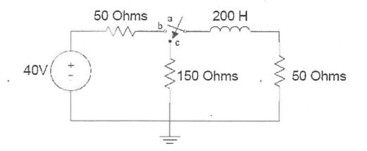
7. Using Matlab programme verify that the maximum power dissipation by the load and Plot the power dissipated by the load.
