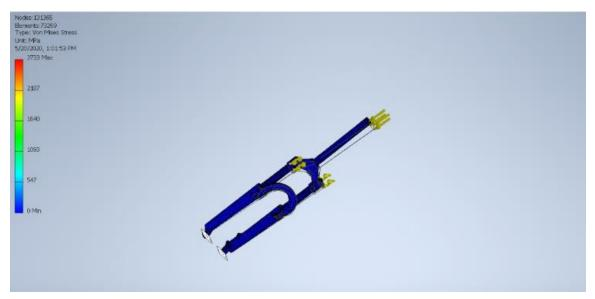
Basic forces were applied on the top and bottom sides of the fork as the bottom holds the tire and the upper part has the weight of the handle.
