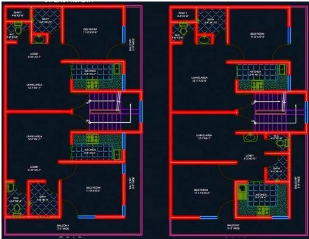
Figure 1. Ground floor and first floor plan of a residential building
