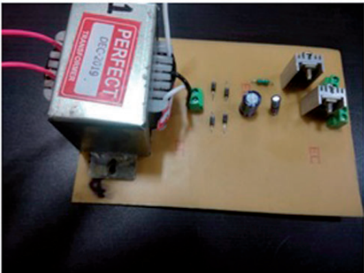
Figure 3. Example of DC power supply made by a group of students, where bridge rectifier is made using 1N 4007 diodes, capacitors, and inductor of specific rating are used to remove ripples in voltage and current, and voltage regulator IC is used for supply voltage regulation.
